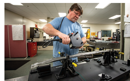
Laser scanning services enables us to achieve quick dimensional accuracy during die design and repair.
