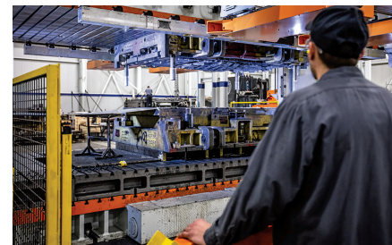
Dies are tried and tested in a production intent environment including feed rates, sensors, and scrap shedding capabilities.
