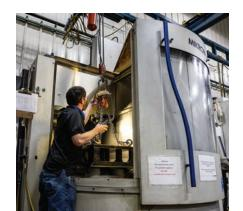
5-axis machining centers with new service packs including advanced controls, drives, spindles, and other internal mechanisms, improving the overall equipment performance.
