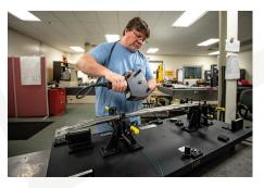
Laser scanning services enables us to achieve quick dimensional accuracy during die design and repair.
