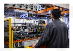
Dies are tried and tested in a production intent environment including feed rates, sensors, and scrap shedding capabilities.
