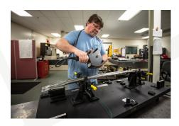
Laser scanning services enables us to achieve guick dimensional accuracy during die design and repair.
