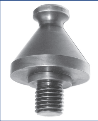
PD500STD – Mega Knob (2 lbs.) Mates with Model 500 Mega Cylinders. Designed to locate large tools and withstand high shear loads. Overall Size: 3.675" H x 2.75" Dia. Knob Height: 2.5625" 1 1/4-7 UNC stud; stud length: 3/4" 1-1/2" Locating Boss: 0.25" H
