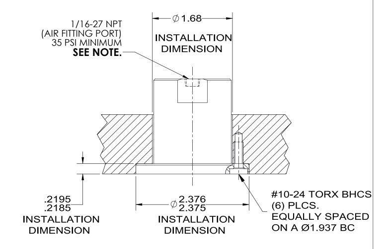
**NOTE:** WHEN INSTALLING 1/16-27 AIR FITTING DO NOT EXCEED TWO FULL REVOLUTIONS. EXCESSIVE FITTING ENGAGEMENT CAN INTERFERE WITH THE CYLINDER LOCKS ABILITY TO ACTUATE PROPERLY, CAUSING IT TO MALFUNCTION!
