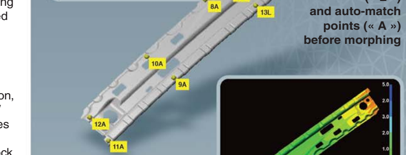
Figure 4 New global deviation after morphing: deviations are twice what they were after applying a 100% compensation factor
